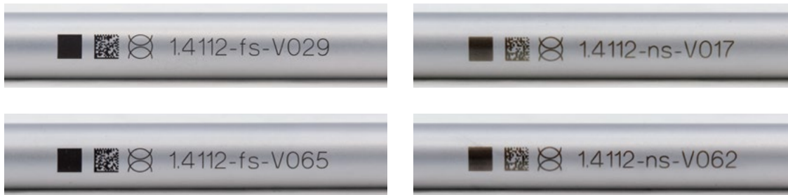
Figure 6: Comparison of annealing markings and black-markings subject to immersion and spray passivation. There are essentially no observable differences in legibility and contrast between the two passivation methods.
