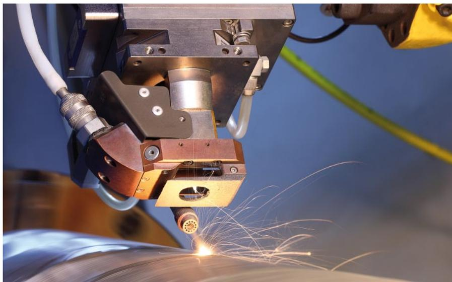
FIGURE 1: Laser cladding using an off-axis nozzle.
