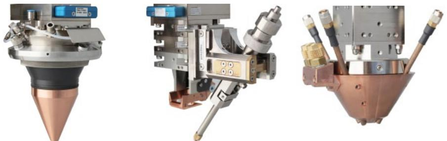
**FIGURE 7:** A choice of powder deposition nozzles enables a full range of components to be cladded with the greatest powder efficiency. The coaxial ring is used for fine detailed work; the four port (discontinuous coaxial) nozzle enables all positional cladding; and the off-axis nozzle is used where process robustness is required, i.e., for beam on times of several hours.
