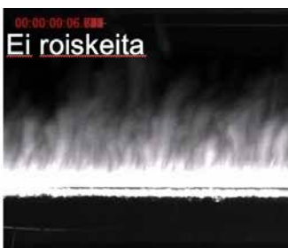
TruDisk – BrightLine Weld LLK 50/200µm, m = 1,5:1, d0 = 75/300µm, P = 1500 W, v = 10 m/min
