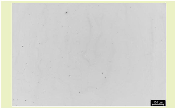
Microsection copper ETP, 100x magnification
