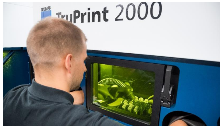
Simply unpack parts in the TruPrint 2000 in an inert atmosphere
