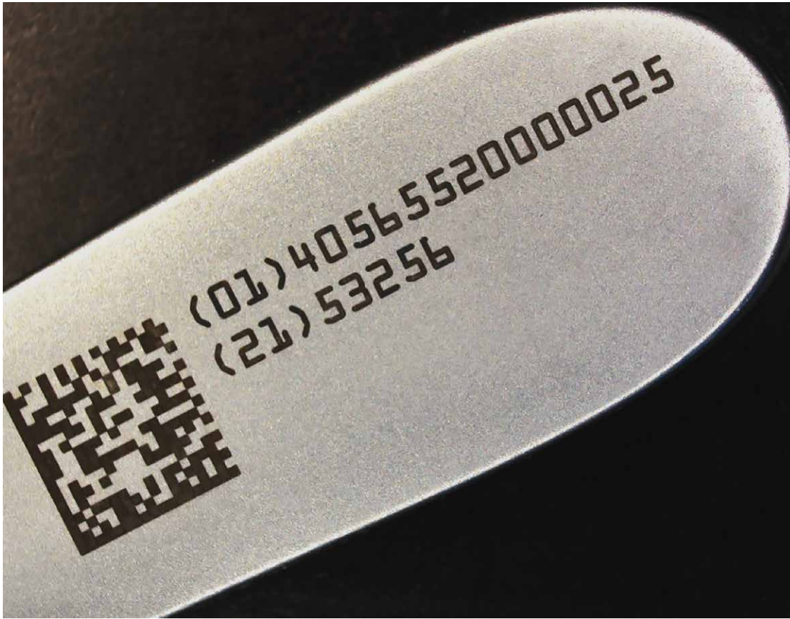
Figure 7: UDI-compliant marking following a 25-hour salt spray test.
