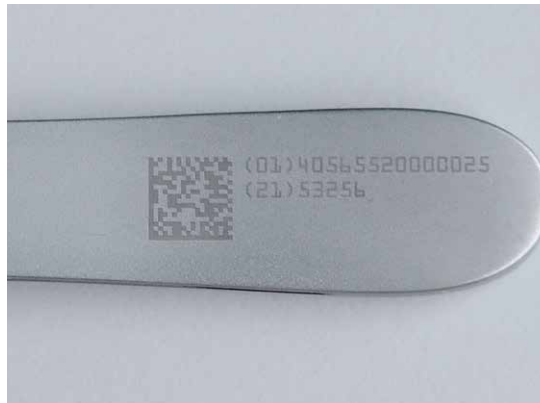
Figure 3: The same marking following a 24-hour salt spray test and 30-minute passivation in citric acid.
