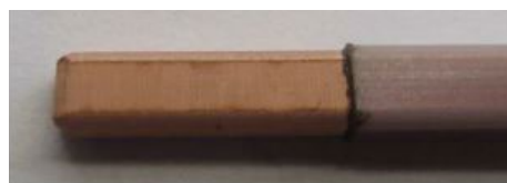
Figure 6: Ablation using a TruMark 7050 machine on a hairpin coated with PEEK. Carbonization effects are visible on the edge.
