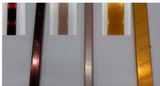
Figure 2: Insulating layers on copper, from left to right: PAI, PEEK, and PAI+FEP.
