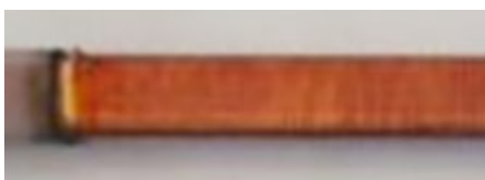
Figure 5: Discoloration on the copper due to the high level of process heat.
