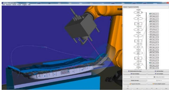
TruTops I-PFO: 3D offline software for the programming of the paths of robots and of scanner programs (I-PFO jobs).
