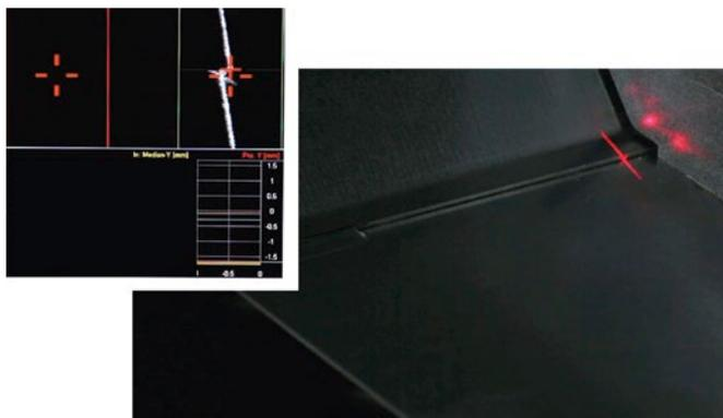
Fillet welding with position control (sensor runs ahead).
