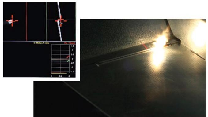
Fillet welding with position control: measurement of target position and actual position during welding.
