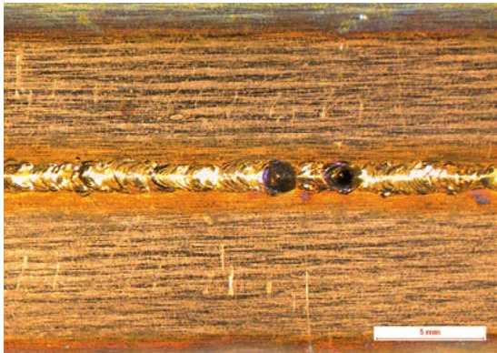
Figure 7: Blowout in a weld seam (top view).
