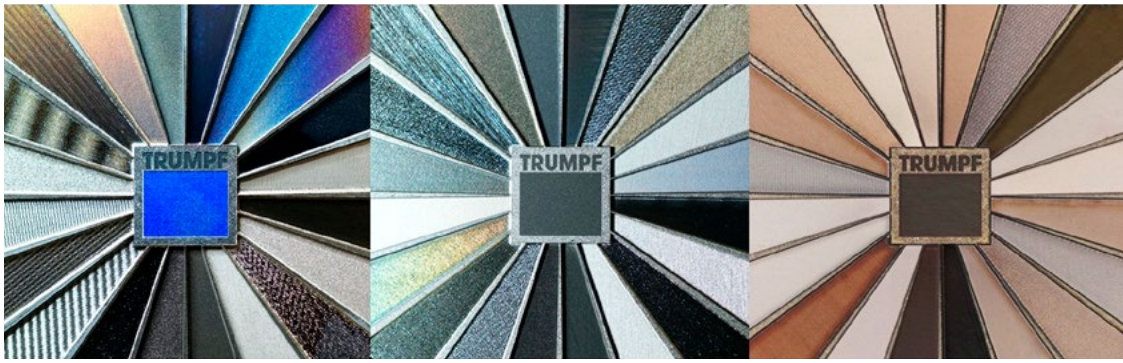
Figure 1: High-quality engraving in titanium (left), 316L (middle) and copper (right). Due to the enormous range of parameters, a wide variety of surface qualities and structures can be achieved by laser engraving with the TruMicro Series 2000.
